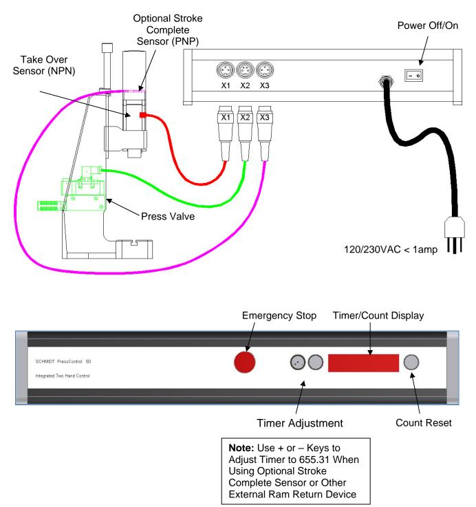
After connections are made, turn power on and insert fingers into the ends of the PC50 to start press cycle.
