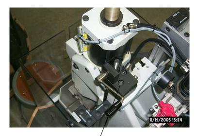
Remove these two screws, so entire height adjustment can be removed with the press.
