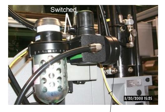
The approach stroke speed can be adjusted via this flow control.
